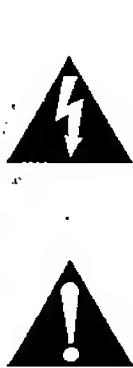
The lightning flash with arrowhead symbol, within an equilateral triangle, is intended to alert the user to presence of uninsulated "dangerous voltage" within the product's enclosure that may be of sufficient magnitude to constitute a risk of electric shock to persons.
